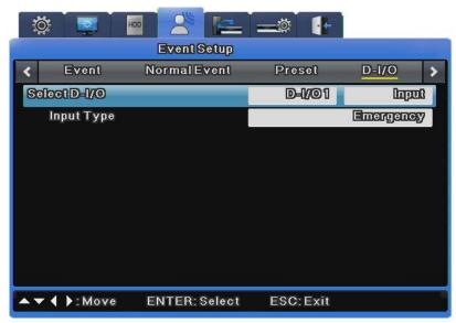
Digital I/O are digital ports available for input and output at the same time., There are 12 digital inputs and outputs.
